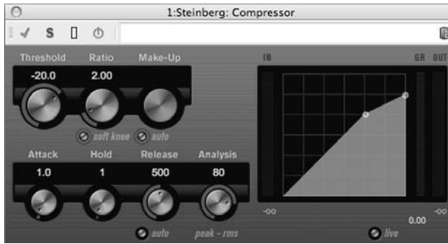
Figure 14.4 The Compressor control panel.
