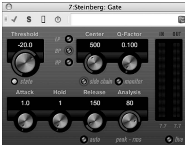
Figure 14.11 The Gate control panel.
