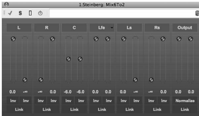
Figure 14.29 The Mix6To2 control panel.
